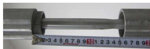
(b) New bolt specimen
