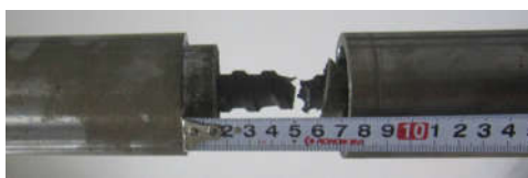
(a) Conventional bolt specimen
