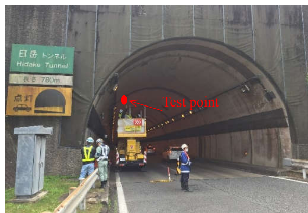
Fig. 3 Ambient vibration test of Hidake Tunnel in Japan
