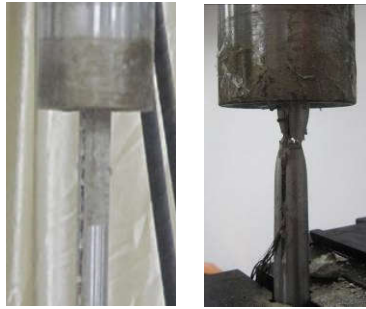
Fig. 11. Different failure modes in the test
