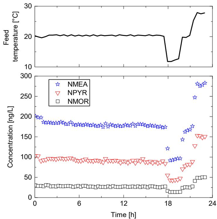
**Fig. S6** – Online analysis of three *N*-nitrosamines (NMEA, NPYR and NMOR) in RO permeate (permeate flux = 20 L/m<sup>2</sup>h, transmembrane pressure = 0.51 MPa). Concentrations of NMEA, NPYR, and NMOR in RO permeate were 900, 990, and 1,040 ng/L, respectively.
