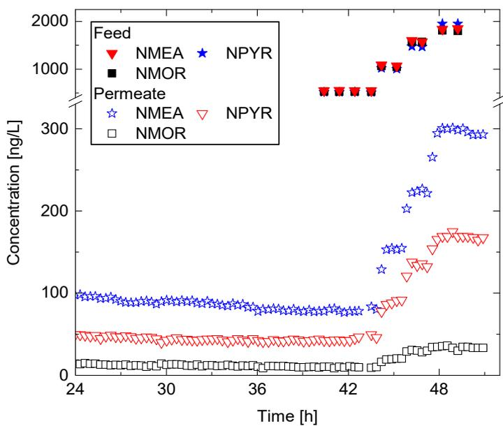
**Fig. S7** – Online analysis of three *N*-nitrosamines (NMEA, NPYR and NMOR) in RO permeate (feed temperature = 20 °C, permeate flux = 20 L/m<sup>2</sup>h, transmembrane pressure = 0.51 MPa). *N*-nitrosamine concentrations in the RO feed were determined based on manual samplings.
