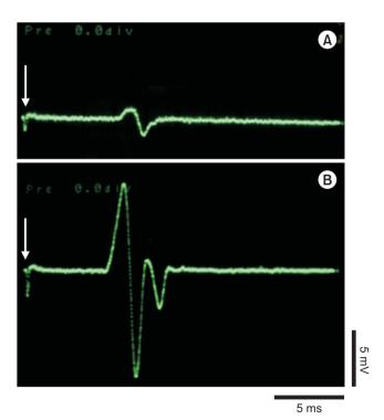
Fig. 1. Oscilloscope photos of jaw opening reflex (JOR) in adult rats. (A) Threshold intensity (101.0  $\mu$ A). (B) 2.5 times threshold intensity (252.5  $\mu$ A). Downward arrows indicate stimulus artifacts.
