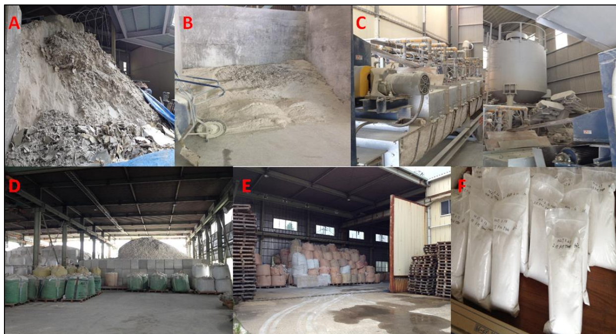
Fig. 1 Waste plaster board recycling process: Crushing and dumping (A) Separation (B) Drying (C) Packing and Recycle (D, E) and Samples after thermal treatment (F)
