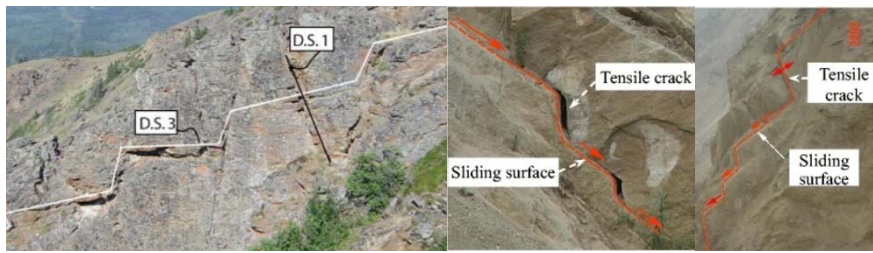
(a) Step-path failure caused by en-echelon fractures [3,4].
