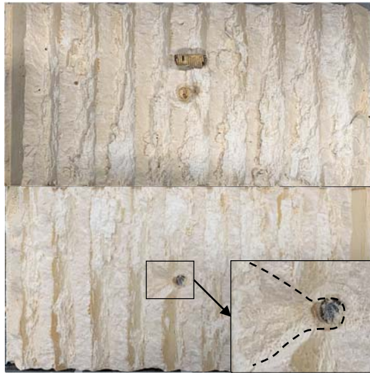
(a) i=-30^\circ Sawtooth failure (Rigid bolt)
