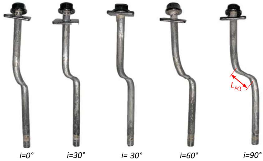
(b) Energy-absorbing bolt
