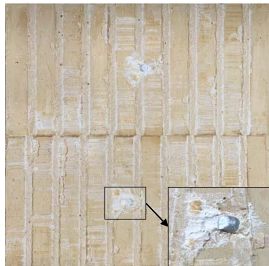
(f) i=0^\circ Planar failure (Energy-absorbing bolt)
