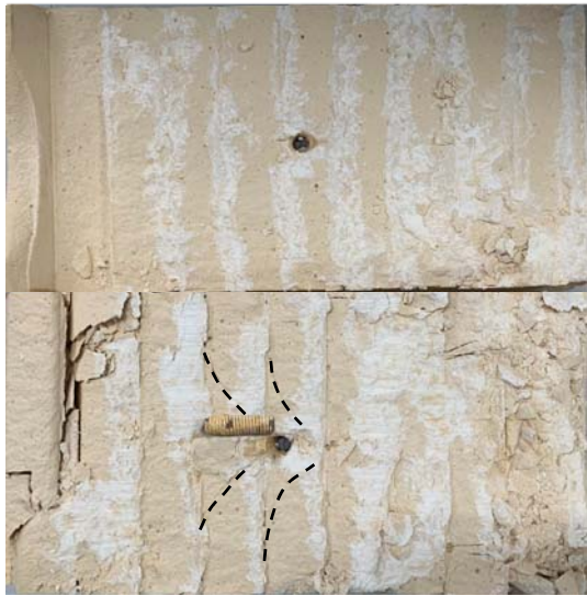
(c) i=60^\circ Block failure (Rigid bolt)
