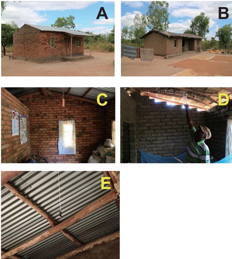
Fig. 1. Typical brick houses in the study sites (A, metal-roof house; B, thatched-roof house), MSRDRD hung from ceiling in the metal-roof house (C) and in the thatched-roof house (D), and a micro data logger (Thermochron® Type G) for measuring room temperature (E).
