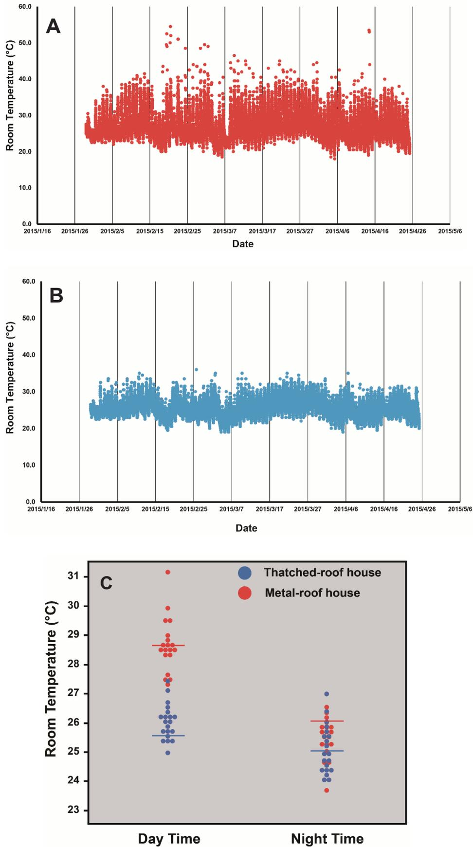
Fig. 2. Changes in the room temperature in metal-roof houses (A) and in thatched-roof houses (B) between January and April, 2015, and average day time (06:00–18:00) and night time (20:00–04:00) room temperature in metal-roof houses and thatched-roof houses (C).
