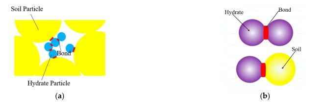
**Figure 5.** Schematic diagram of hydrate sediment contact model: (**a**) cemented cluster hydrate sediments; (**b**) schematic diagram of 3D cementation model.
