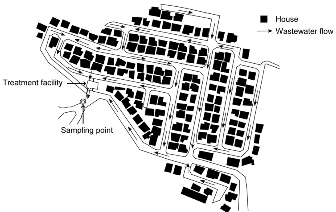
Fig. 3.3 Site 6 showing the flow of untreated household effluents, the treatment facility and the sampling point.
