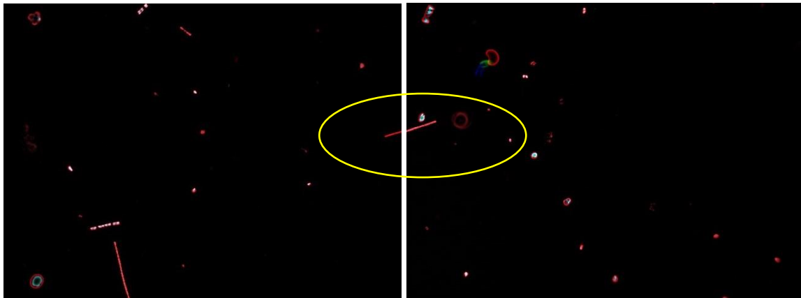
Fig 4.10 A filament of Pseudanabaena sp. on two consecutive microscopic images in fluorescence observation: the single Pseudanabaena sp. was counted as two units with the developed auto-counting technique.
