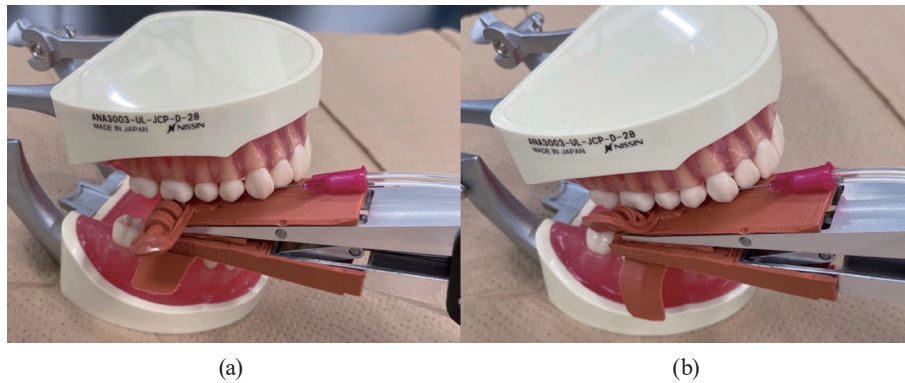
Fig. 6. (Color online) Silicone tip connected to the negative pressure device: (a) normal state and (b) under negative pressure.
