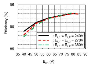
Fig. 6. Power efficiency against change of output voltage in parallel operation at  $I_{\text{oR}} = 160 A$
