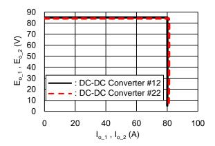
Fig. 5. Characteristics of dc-dc converters #12 and #22
