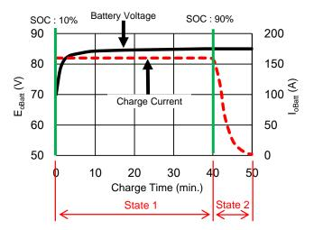
Fig. 8. Charging characteristics of battery
