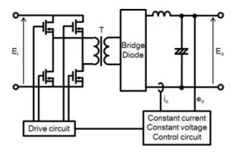
Fig. 3. Block diagram of dc-dc converter
