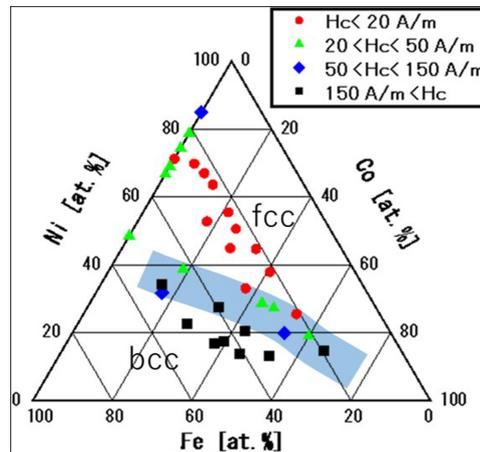
FIG. 4. Ternary diagram for the coercivity of the Fe-Co-Ni films.
