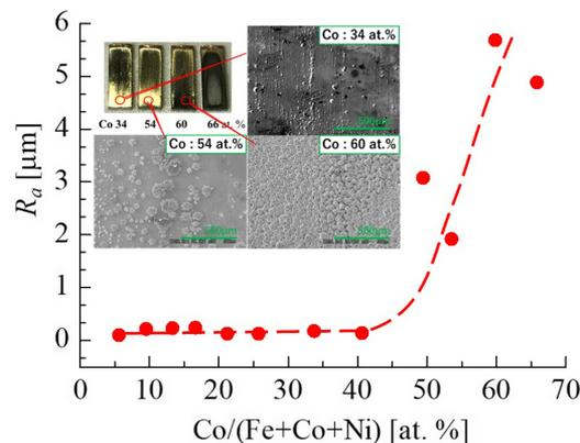
FIG. 2. The surface roughness of the as-plated Fe-Co-Ni films as a function of the Co content in the film. The insets indicate photographs and SEM images for some Fe-Co-Ni films.
