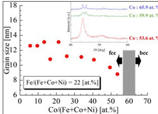
FIG. 3. The grain size of the as-plated Fe-Co-Ni films as a function of amount of the Co content in the films. The insets indicate XRD patterns for the Fe-Co-Ni films with high Co content.
