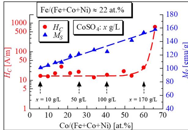
FIG. 1. The coercivity and the saturation magnetization of the as-plated Fe-Co-Ni films as a function of the Co content in the films.
