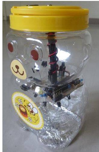
Fig. 2.12 Developed infrared controller in a bear shape bottle
