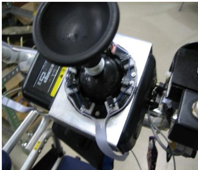
Fig. 4.8 Joystick with eight limit-switches
