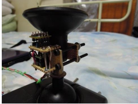
Fig. 4.3 Joystick with acceleration and gyro-sensor
