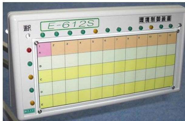
Fig. 1.10 Environmental control system (E-612S)[9]
