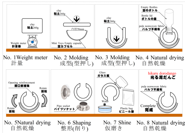
Fig. 2 Manufacturing procedure for spherical mud balls (SDGs Shiny Mud Balls) consisting of hollow and shell with a thickness of several millimeters
