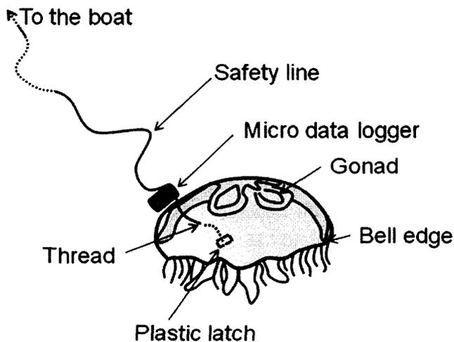
Fig.2 Schematic diagram of the micro data logger attached to the moon jelly.
