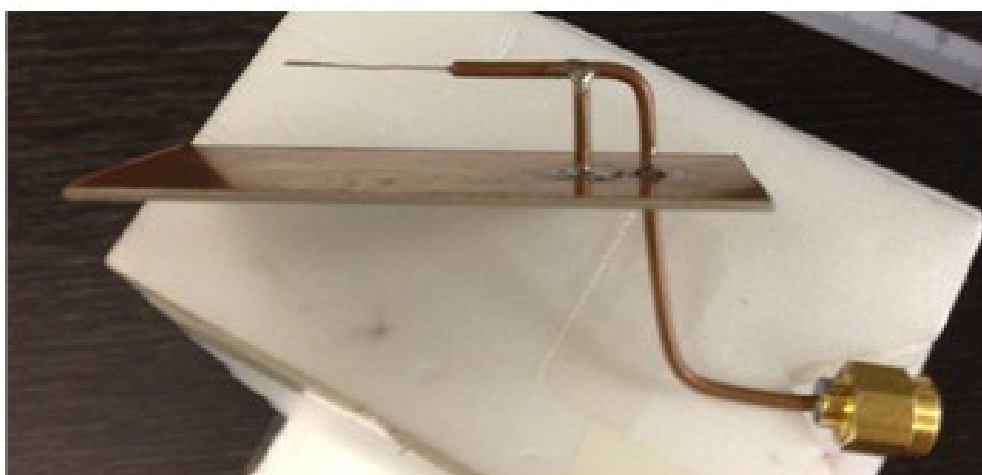
Fig. 4.4a. The photograph of fabricated ULPIF antenna ( h=10\text{mm} , L_s=6.6\text{mm} , L1+L_s=17.1\text{mm} , L+L_s=34.1\text{mm} , p_{xp}=p_{xm}=15\text{mm} , p_{ym}=16.8\text{mm} , p_{yp}=43.2\text{mm} ).
