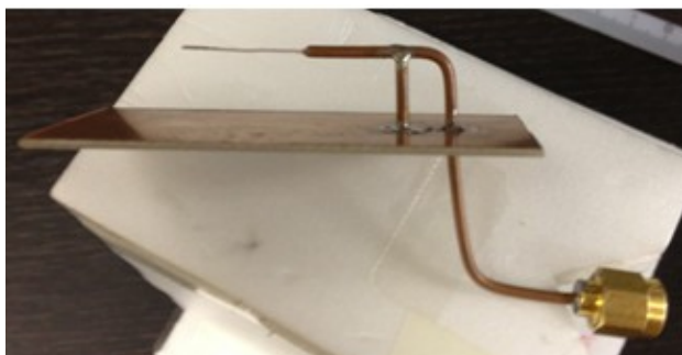
Fig. 4a. The photograph of fabricated ULPIF antenna ( h=10\text{mm} , L_s=6.6\text{mm} , L_1+L_s=17.1\text{mm} , L+L_s=34.1\text{mm} , p_{xp}=p_{xm}=15\text{mm} , p_{ym}=16.8\text{mm} , p_{yp}=43.2\text{mm} ).
