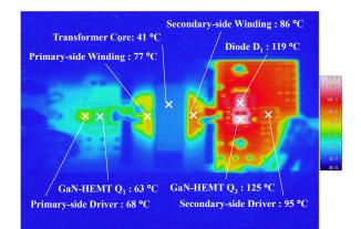
Fig. 13. The temperature distribution that temperature region is from 20°C to 130°C of resonant DC-DC converter with the proposed PWM control method at M = 1.05,  $I_o = 10$ A, D = 0.59.
