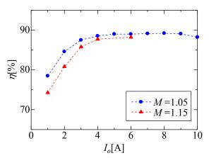
Fig. 12. The power efficiency of resonant DC-DC converter with the proposed PWM control method.
