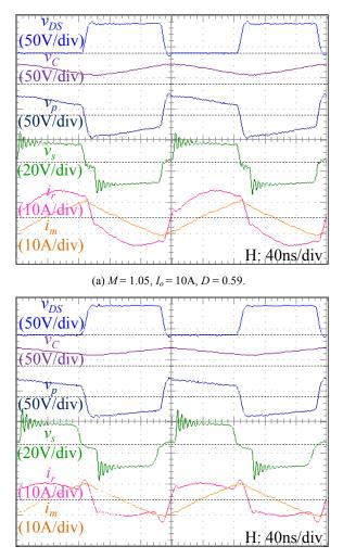
(b) M = 1.15,  $I_o = 6A$ , D = 0.63. Fig. 11. Experimental waveforms of resonant DC-DC converter with the proposed PWM control method.
