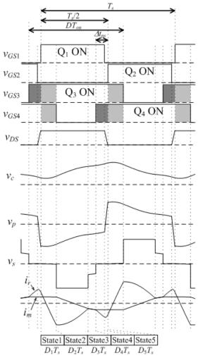
Fig. 4. The operational waveforms of the proposed PWM control.
