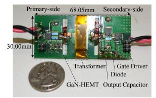
Fig. 9. The prototype of the DC-DC converter.
