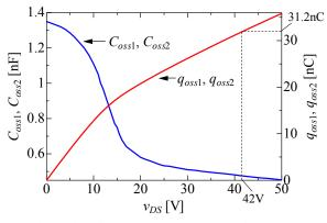
Fig. 6. The influence of  $v_{DS}$  on  $C_{oss1}$ ,  $C_{oss2}$  and  $q_{oss1}$ ,  $q_{oss2}$ .
