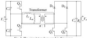
Fig. 3. The circuit topology used in this paper.
