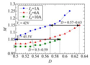
Fig. 10. The open loop static characteristics of resonant DC-DC converter with the proposed PWM control method.
