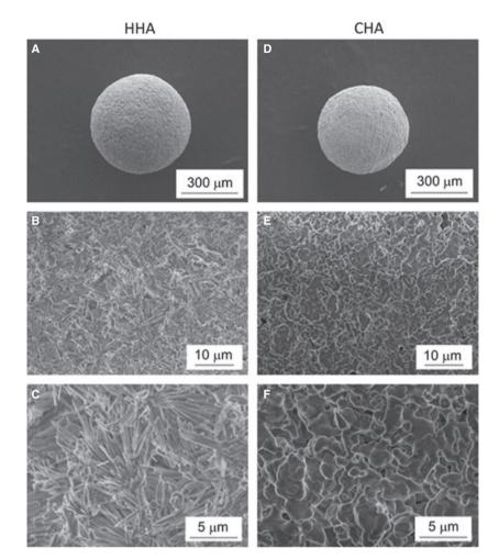
Fig. 1 Scanning electron micrographs of the overview (A and D) and the microstructure (B, C, E and F) of HHA (A–C) and CHA (D–F) granules.
