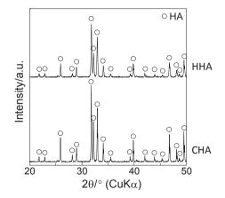
Fig. 2 X-ray diffractometry (XRD) of implants used in this study. From XRD patterns, the main phases of HHA and CHA were assigned to HA.
