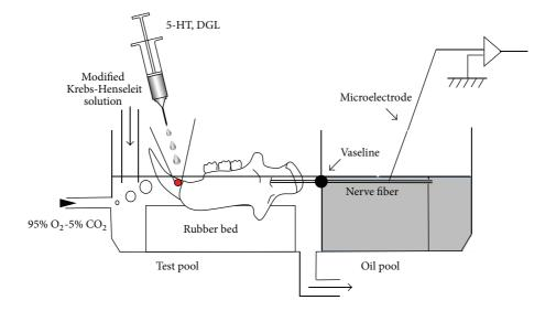
FIGURE 1: Schematic presentation of the chamber setup for the *in vitro* jaw-nerve preparation (see text for details).
