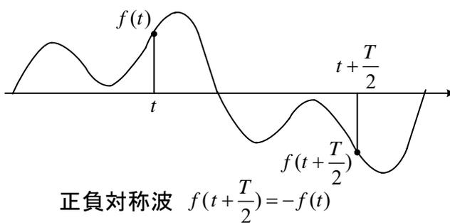
$$f(t + \frac{T}{2}) = a_0 + \sum_{n=1}^{\infty} \left\{ a_n \cos(n\omega_0 t + \frac{n\omega_0 T}{2}) + b_n \sin(n\omega_0 t + \frac{n\omega_0 T}{2}) \right\}$$
