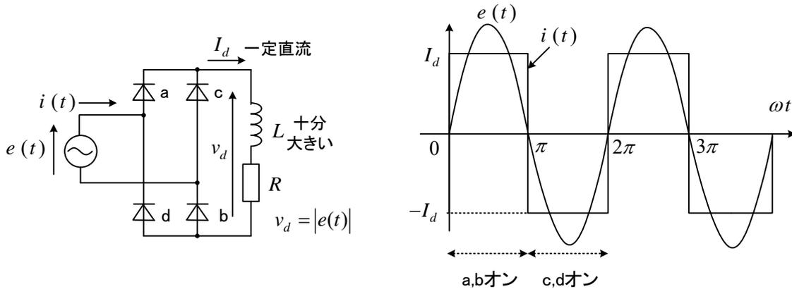
(解) (1)  $I_e = \sqrt{\frac{1}{T} \int_0^T i^2 dt} = \sqrt{\frac{1}{T} \int_0^T I_d^2 dt} = I_d$       ここで、周期  $T = \frac{\omega}{2\pi}$
