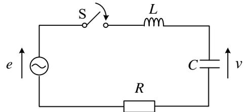
(答)  $v(t) = V_m \sin(\omega t + \varphi - \theta) - V_m \sin(\varphi - \theta) e^{-\alpha t} \cos \beta t$
