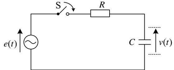
(答)  $v(t) = \frac{E_m}{\sqrt{1+(\omega CR)^2}} \left\{ \sin(\omega t + \varphi - \theta) - e^{-\frac{t}{RC}} \sin(\varphi - \theta) \right\}$  ただし、 $\theta = \tan^{-1}(\omega CR)$
