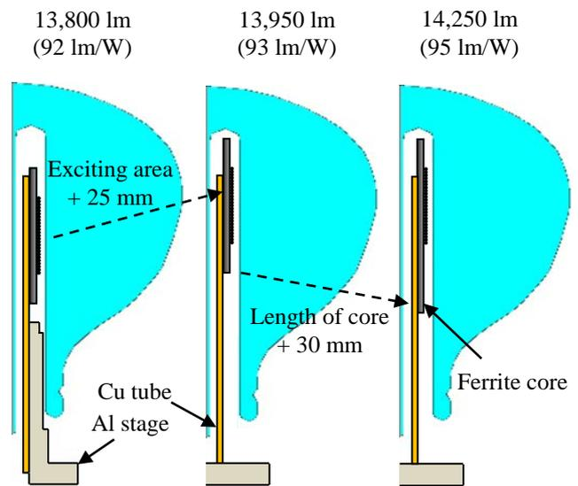
Fig. 7 Schematic representation of the coupler in the measured lamp. Measured values of the luminous flux and the lamp efficiency are also shown in the top of each lamp.
