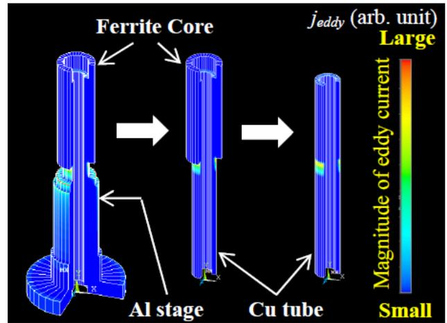
Fig. 2 Eddy current per unit volume in the power coupler of the commercial lamp.
