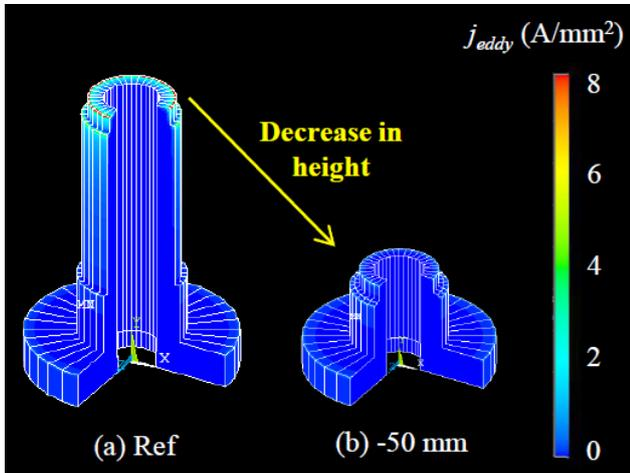
Fig. 4 Contour figure for eddy current per unit volume in the Al stage before and after reducing the height.
