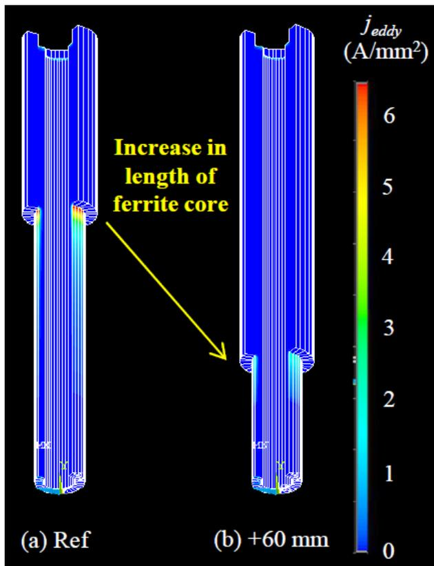
Fig. 5 Contour figure for eddy current per unit volume in the Cu tube before and after elongation of the core.
