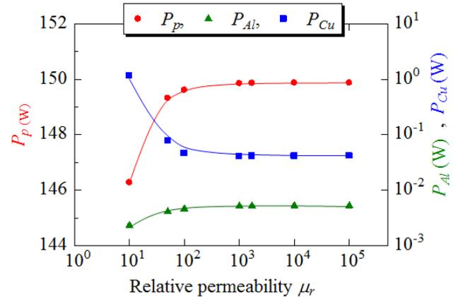
Fig. 6 Change in eddy current loss in plasma  $P_p$ , Cu tube  $P_{Cu}$  and Al stage  $P_{Al}$  as a function of the relative permeability of the ferrite core. The relative permeability for a commercial lamp is 1700.
