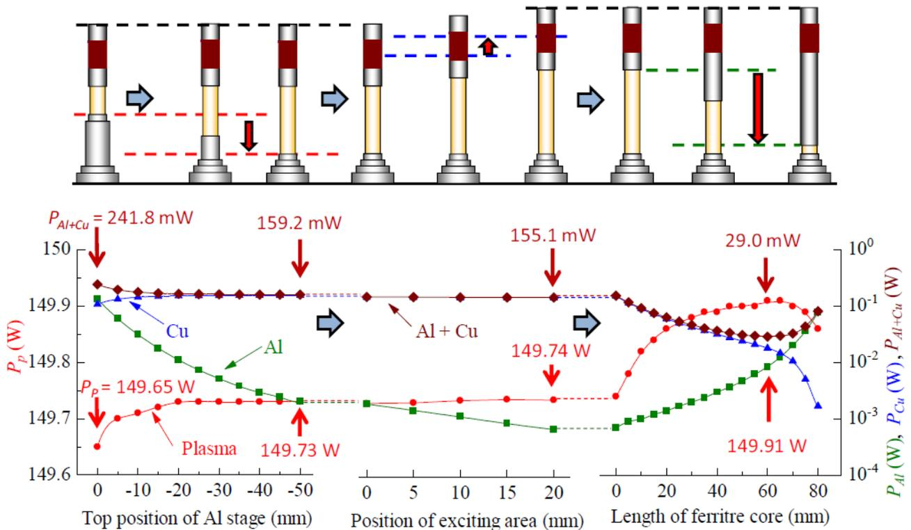
Fig. 3 Eddy current losses of the Al stage  $P_{Al}$  and the Cu tube  $P_{Cu}$  calculated with various simulation models. The simulation models are shown in the same figure schematically. Calculated eddy current loss of the plasma  $P_p$  is also shown as a reference.
