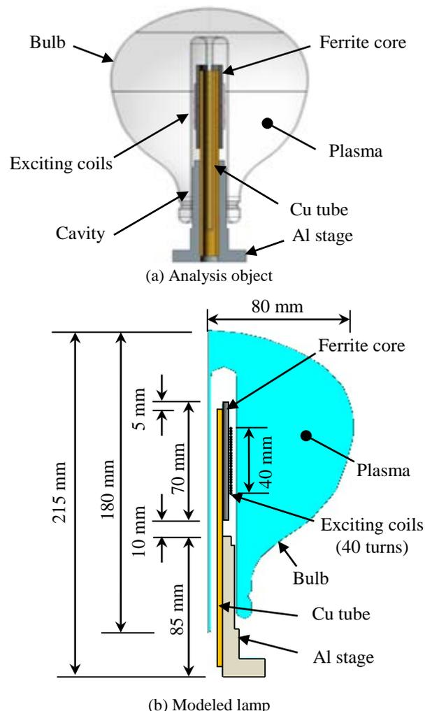
Fig. 1 Analysis objects and modeling of a lamp. A spherical electrodeless discharge lamp (150 W type) produced by Panasonic Ltd. is used as reference model in this study.
