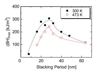
FIG. 7.  $(BH)_{\rm max}$  of isotropic SmCo<sub>5</sub>/ $\alpha$ -Fe nanocomposite magnets at 300 K and 473 K as a function of the stacking period,  $t_{\rm s}$ . The averaged values for 5 model magnets are shown in the Figure.
