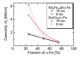
FIG. 2. Coercivity of anisotropic SmCo<sub>5</sub>/ $\alpha$ -Fe nanocomposite magnets at 300 K as a function of  $\alpha$ -Fe fraction, together with results for Nd<sub>2</sub>Fe<sub>14</sub>B/ $\alpha$ -Fe ones. The stacking periods were set at 8 and 16 nm.
