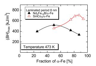
FIG. 4.  $(BH)_{max}$  of anisotropic SmCo<sub>5</sub>/ $\alpha$ -Fe nanocomposite magnets at 473 K as a function of the fraction of  $\alpha$ -Fe together with results for Nd<sub>2</sub>Fe<sub>14</sub>B/ $\alpha$ -Fe ones. The stacking period was set at 8 nm.
