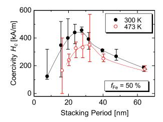
FIG. 5. Coercivity  $H_c$  of isotropic SmCo<sub>5</sub>/ $\alpha$ -Fe nanocomposite magnets at 300 K and 473 K as a function of the stacking period,  $t_s$ . The averaged  $H_c$  values for five models and error bars were shown in the figure. The thickness ratio of  $\alpha$ -Fe to SmCo<sub>5</sub> layers was set at 1.
