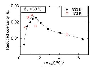
FIG. 6. Reduced coercivity,  $h_c (= H_c/H_A)$ , as a function of  $\eta (= J_h S/K_u V)$ , where  $K_u$  and  $K_A$  are the magnetic anisotropy constant and anisotropy field of SmCo<sub>5</sub>, and S and V are the surface area and volume of a grain. Furthermore,  $J_h$  is the exchange constant of SmCo<sub>5</sub>. The explanation about  $\eta$ is in the text.
