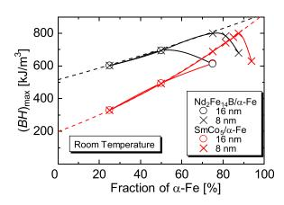
FIG. 3.  $(BH)_{max}$  of anisotropic SmCo<sub>5</sub>/ $\alpha$ -Fe nanocomposite magnets at 300 K as a function of  $\alpha$ -Fe fraction together with results for Nd<sub>2</sub>Fe<sub>14</sub>B/ $\alpha$ -Fe ones. The stacking periods were set at 8 and 16 nm.
