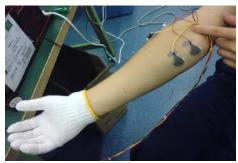
Fig.3 The myoelectric sensors
