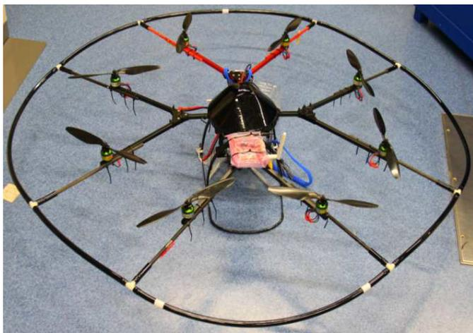
Fig. 1. Disk-type flying robot
