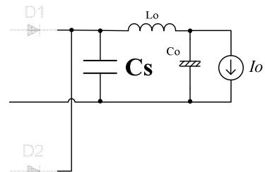
Fig.11. Equivalent circuit during the dead time
