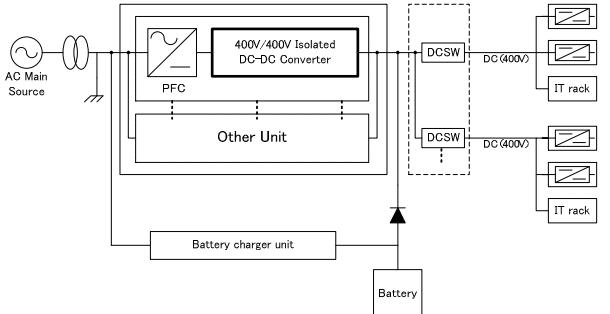
Fig.1. Block diagram of HVDC power distribution system with PFC converter and 400V/400V isolated DC-DC converter.
