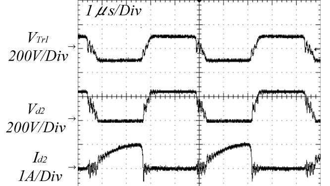
Fig.6. Experimental waveforms of surge occurrence (with snubber capacitance  $C_s=1.1\mu F$ ).
