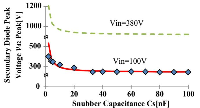
Fig.13. Effect of snubber capacitance on diode's surge voltage.
