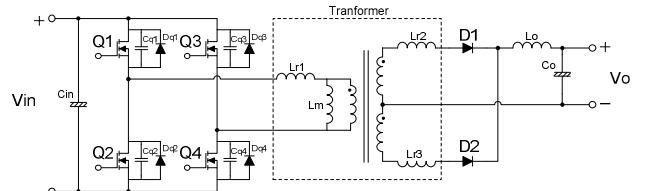
Fig.2. Circuit topology of full-bridge isolated DC-DC converter
