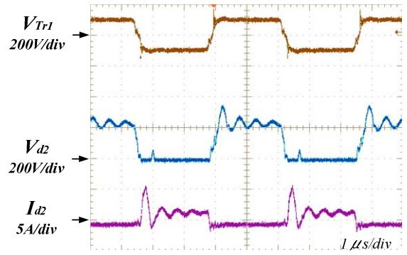
Fig.7. Experimental waveforms of surge occurrence (with snubber capacitance  $C_s=5\text{nF}$ )
