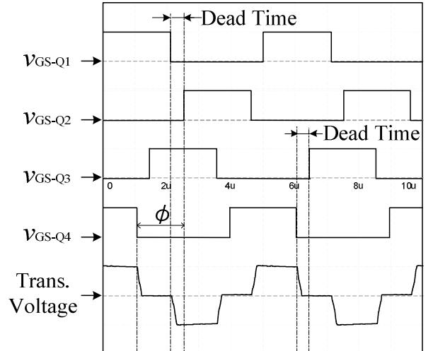
Fig.14. Gate-voltage pattern of primary switches Q1-Q4 for phase-shift control.
