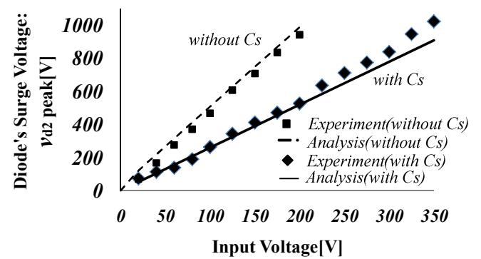
Fig.12. Analytical and experimental results for diode's surge voltage
