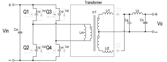
Fig.8. Circuit state during the dead time
