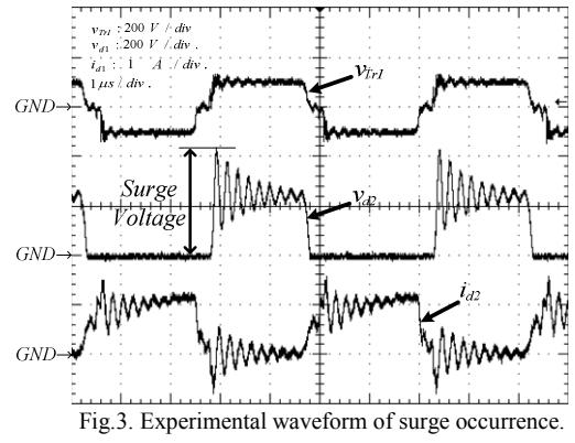
Fig.3. Experimental waveform of surge occurrence.
