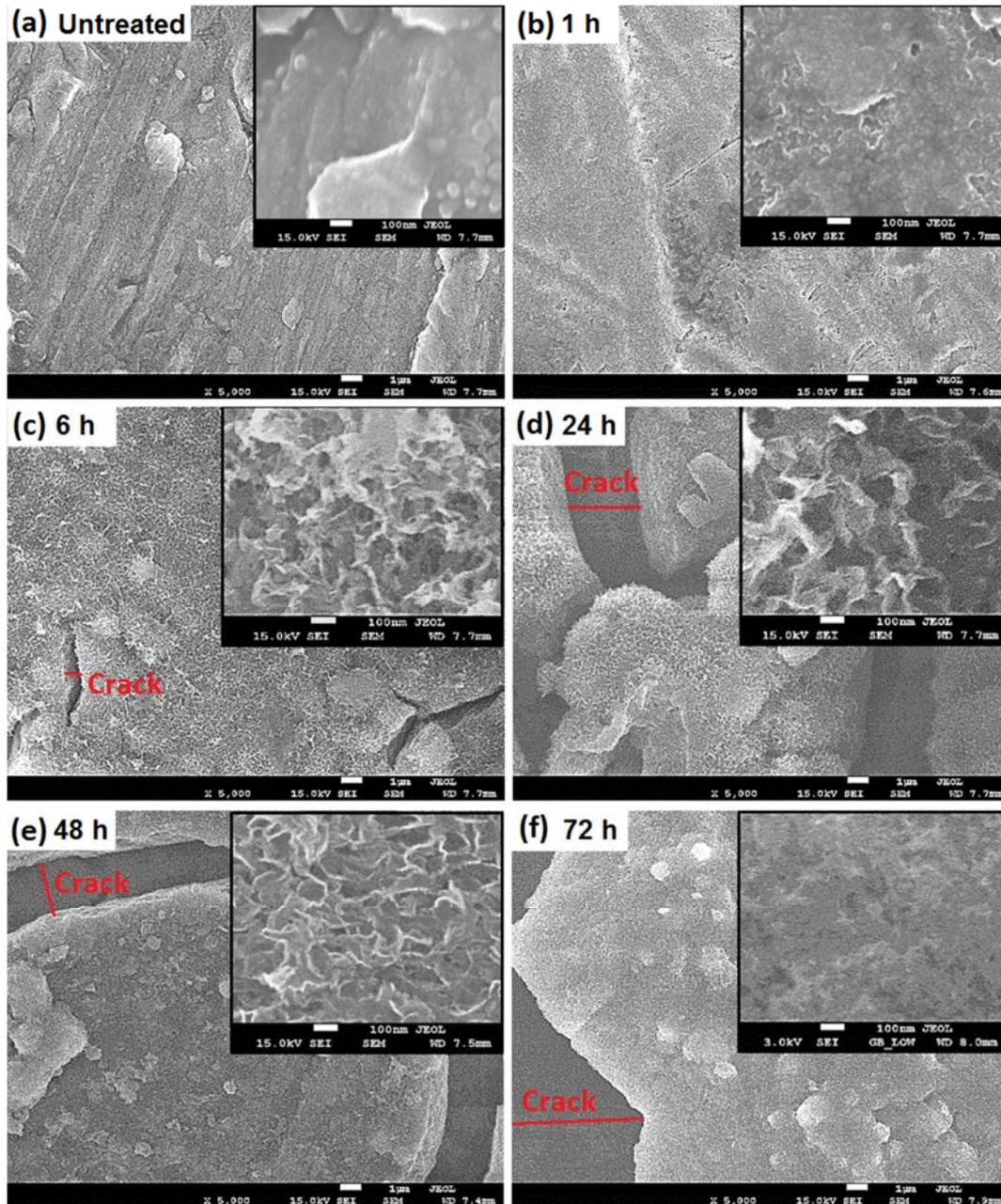
Fig. 1. FESEM micrographs of the untreated and treated titanium samples at different treatment times: (a) untreated; (b) 1 h; (c) 6 h; (d) 24 h; (e) 48 h; (f) 72 h.
