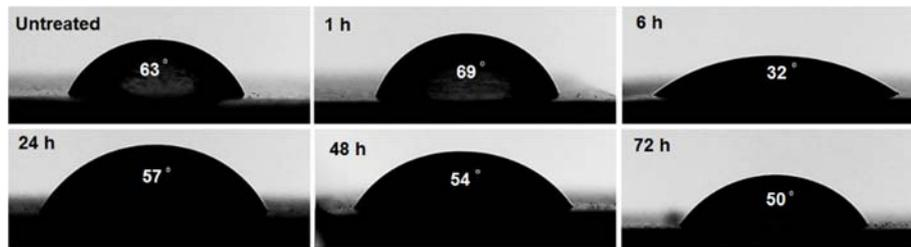
Fig. 4. Water contact angles of the untreated and treated titanium samples at different times.
