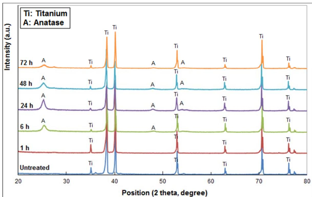
Fig. 2. X-ray diffraction patterns of the untreated and treated titanium samples at different times.
