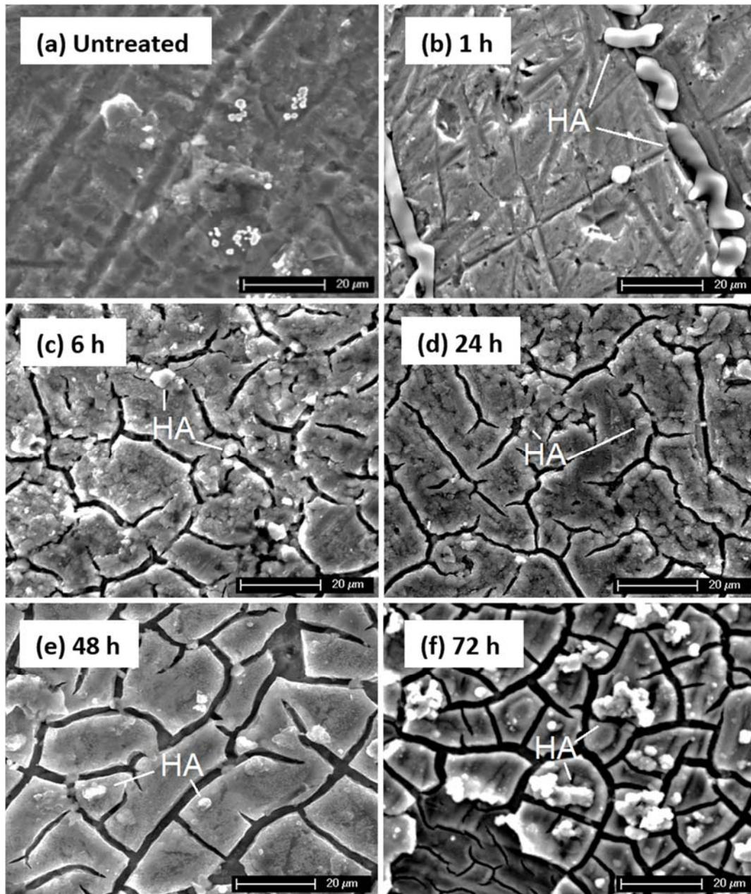
Fig. 5. Bone-like apatite formation on the surface of untreated and treated titanium samples at different times (after 7 d of immersion in SBF): (a) untreated; (b) 1 h; (c) 6 h; (d) 24 h; (e) 48 h; (f) 72 h.
