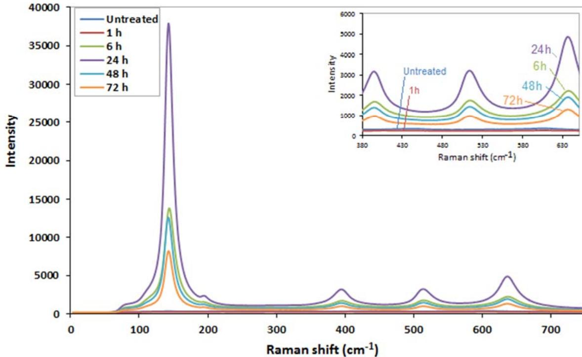
Fig. 3. Raman spectras of the untreated and treated titanium samples at different times.
