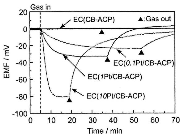
Figure 2. Response transients of EC( $n$ Pt/CB-ACP) and EC(CB-ACP) to 500 ppm CO in air at 30°C (57%RH).
