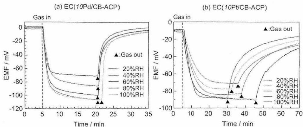
Figure 5. Response transients of EC(10Pd/CB-ACP) and EC(10Pt/CB-ACP) to 500 ppm CO in air at 30°C (20~100%RH).
