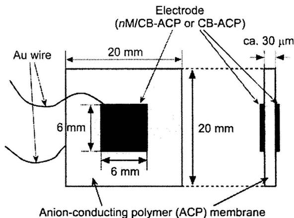
Figure 1. Schematic drawing of a sensor element.
