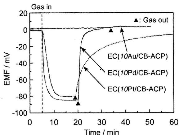
Figure 3. Response transients of EC(10M/CB-ACP) to 500 ppm CO in air at 30°C (57%RH).
