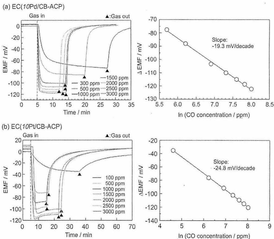
Figure 4. Response transients to CO and CO concentration dependence of response of EC(10Pd/CB-ACP) and EC(10Pt/CB-ACP) in air at 30°C (CO concentration: 100~3000 ppm, 57%RH).
