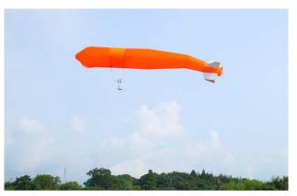
Fig. 15. Balloon type flying robot.
