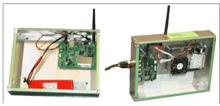
Fig. 3. Video data transmitting unit.
