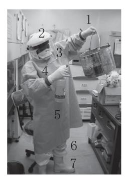
Fig. 6. P3 Lab user in full PPEs. 1: Gloves (double), 2: Face Shield, 3: N95 mask, 4: Wrist band, 5: Front covered gown, 6: Coverall, 7: Safety boots
