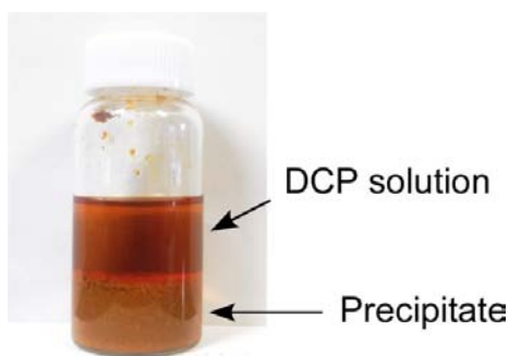
Figure 1. Photograph of precipitate deposited after the mixing of the ACP solution and the electrolyte solution.
