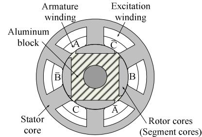
Figure 1. Construction of segment type RG and SRG
