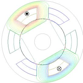
Figure 3. Magnetic flux on the aligned position (angle: 30deg)
