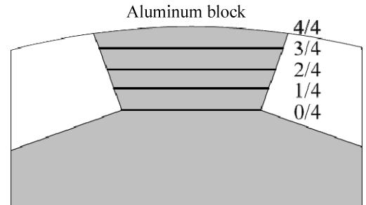
Figure 9. Definition of the aluminum height
