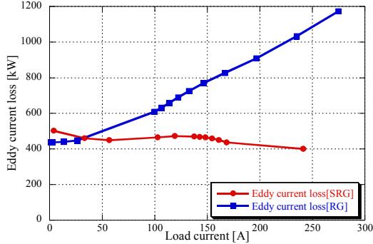
Figure 8. Characteristics of the eddy current loss
