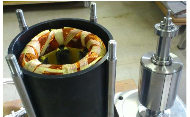
Figure 12. The 2kW segment type SRG
