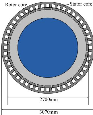
Figure 5. SRG full model (stator: 48 poles)
