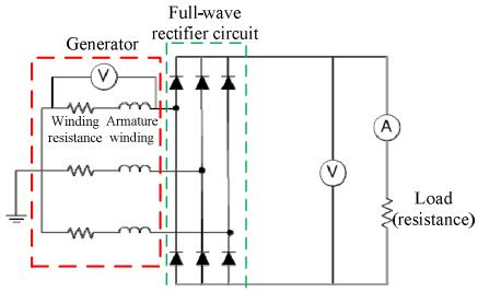
Figure 4. External circuit (load side)
