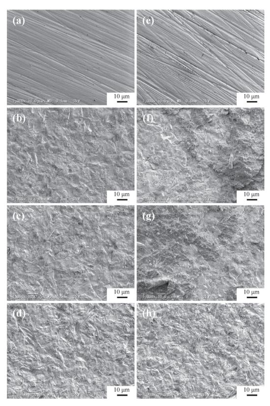
Fig. 2 Scanning electron micrographs of representative thermally cycled and debonded compositezirconia fracture surfaces:
