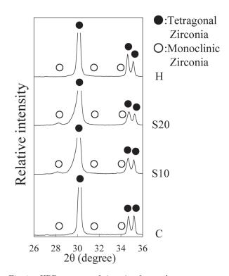
Fig. 1 XRD patterns of zirconia after each treatment.
