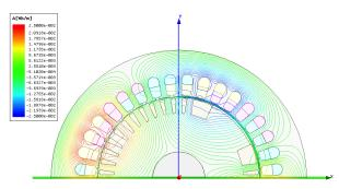
(d) Magnetic flux distribution produced by armature current at  $\omega t=60^{\circ}$ .
