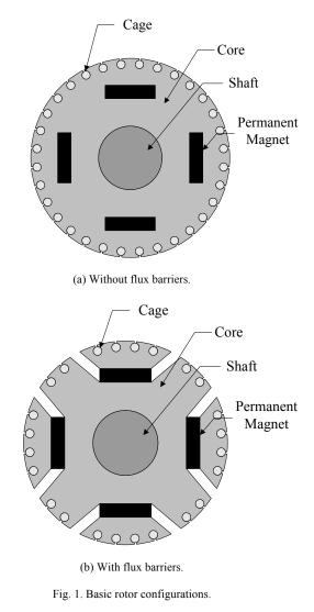
We propose a rotor configuration for a line-start permanent magnet synchronous motor to produce both the performances. The rotor contains the permanent magnets mounted on the surface and squirrel cage windings. This paper describes the detailed explanation of the proposed motor and shows the fundamental characteristics of the line-start permanent magnet synchronous motor with the rotor.
