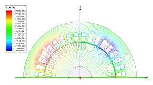
(c) Magnetic flux distribution produced by armature current at  $\omega t=0^{\circ}$ .
