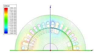
(e) Magnetic flux distribution produced by armature current at  $\omega t=120^{\circ}$ .
