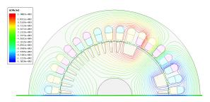
(b) Magnetic flux distribution produced by magnets.
