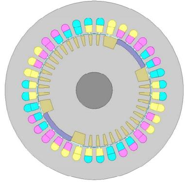
Fig. 3. 2-dimensional model of self-start type PMSM.
