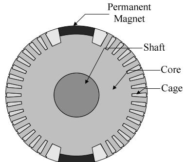
Fig. 2. Rotor of self-start type PMSM
