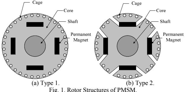
Fig. 1. Rotor Structures of PMSM.
