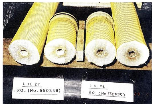
Fig. 5. Sections of dirty module.
