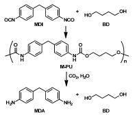
We have demonstrated a hydrolysis reaction of polyurethane (M-PU) under high pressure of carbon dioxide (CO<sub>2</sub>) in water. The optimum hydrolysis reaction condition was 190 °C under CO<sub>2</sub> pressures over 4.1 MPa in water medium, and 93% hydrolysis of M-PU was achieved. This hydrolysis under high pressure of CO<sub>2</sub> with water is a reaction by which M-PU is selectively hydrolyzed into consisted chemicals of repeating units of M-PU by cleaving urethane linkage.
