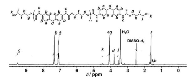
**Figure 2**. <sup>1</sup>H-NMR spectrum of residual water-insoluble parts (hydrolyzed M-PU) in DMSO-*d*<sub>6</sub>.
